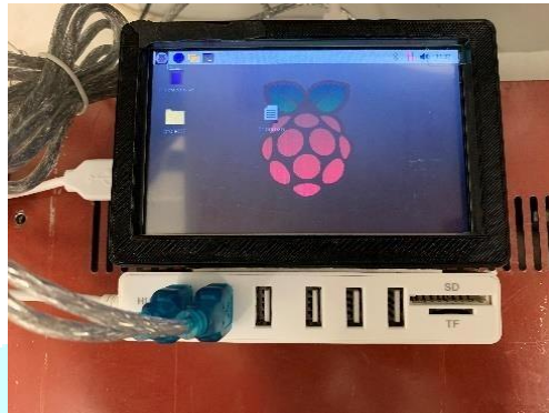
Fig.6. The Raspberry-Pi is connected to instruments via USB ports and stored in a 3-D printed box (designed using Open-Scad)
