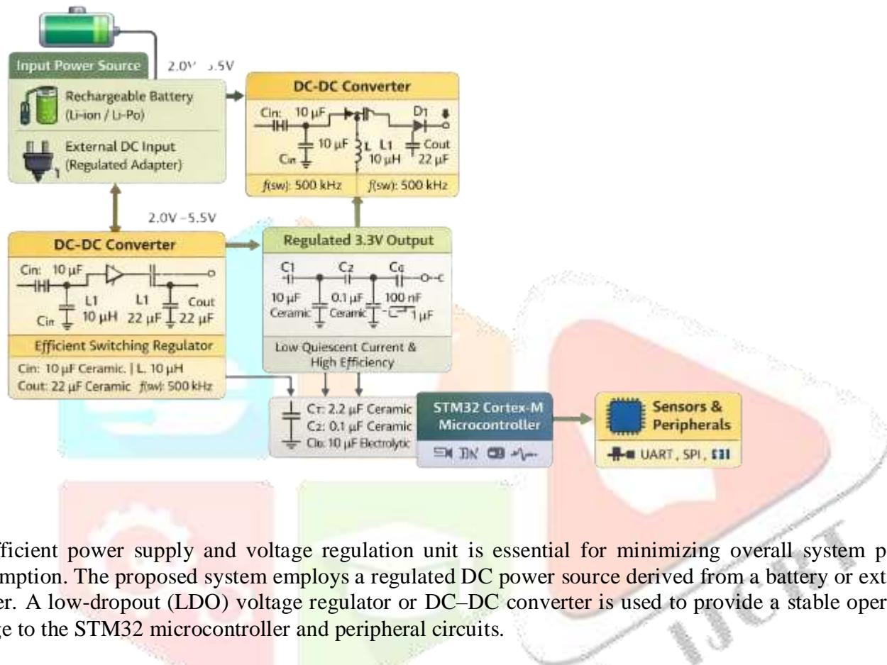
An efficient power supply and voltage regulation unit is essential for minimizing overall system power consumption. The proposed system employs a regulated DC power source derived from a battery or external adapter. A low-dropout (LDO) voltage regulator or DC-DC converter is used to provide a stable operating voltage to the STM32 microcontroller and peripheral circuits.
