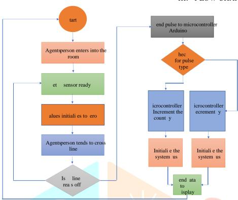
The operation of the system is already been discussed in previous section. In this section we will discussed about the flowchart that how it works. So above flowchart shows that the system iterates for infinite times until and unless the system is switched OFF or power cut. This is because the LDR sensors after break off, automatically adjusted to go to previous state that is the LDR line is again connected in each sensor set. The pseudo codes for the operation are shown below:
