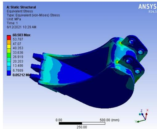
Fig.12: Equivalent Stresses of Excavator Bucket
