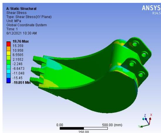
**Fig.11: Shear Stress due to loading on Excavator Bucket**
