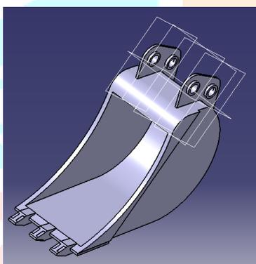
Fig.6: CAD model of Bucket
