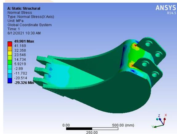
Fig.13: Normal Stress Value obtained for Excavator Bucket
