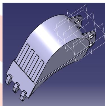
Fig.7: CAD model of Bucket
