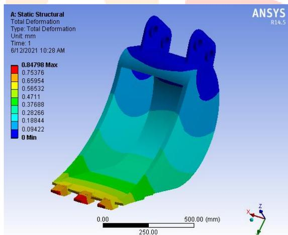
**Fig. 10: Total Deformation in excavator bucket**
