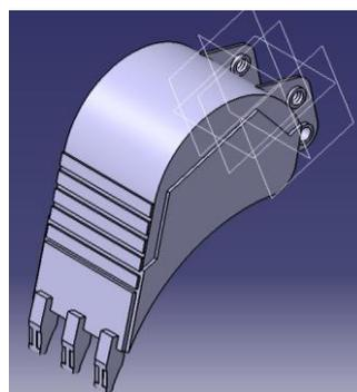
Fig.5: CAD model of Bucket
