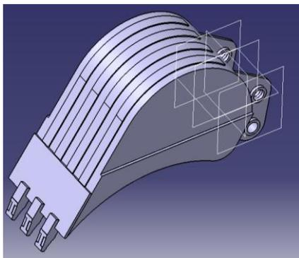
**Fig. 3:** CAD model of Bucket
