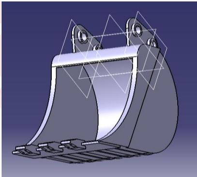
**Fig. 2:** CAD model of Bucket
