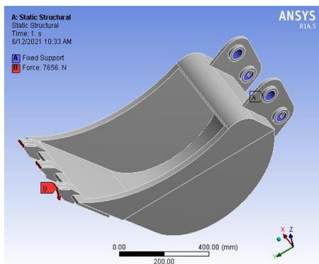
**Fig.9: Forces Applied on Excavator Bucket**
