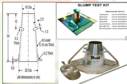
FIGURE.3 - DETAILS OF SLUMP FLOW APPARATUS
