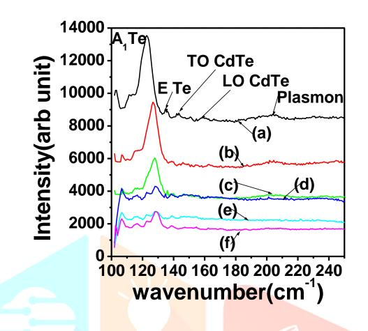
Figure 2. Micro Raman studies: (a) Pristine, (b)  $1.0 \times 10^{11}$ , (c)  $5.0 \times 10^{11}$ , (d)  $1.0 \times 10^{12}$ , (e)  $5.0 \times 10^{12}$ , (f)  $1.0 \times 10^{13}$  cm<sup>-2</sup>
