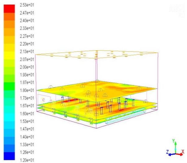
Fig.25: Contours of Relative Humidity for Case 2.
