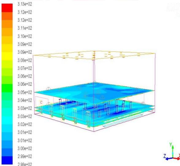
Fig.24: Contours of static Temperature for Case 2.
