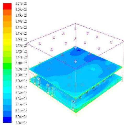
**Fig.20: Contours of static Temperature for Event Case1.**
