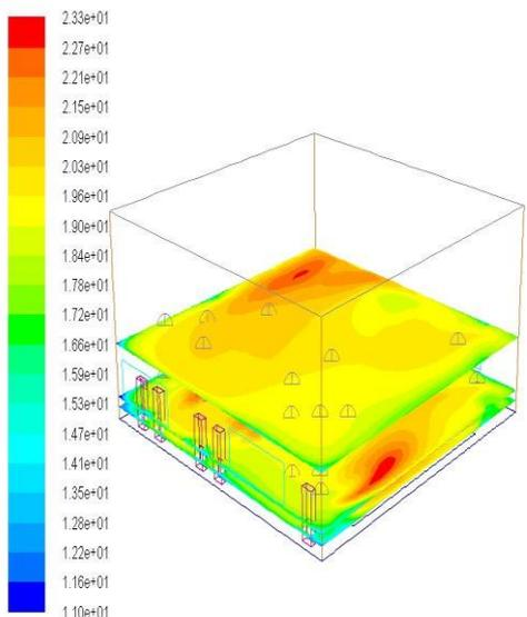
**Fig.18: Contours of Relative Humidity for Cooling Case1.**
