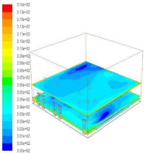
**Fig.17: Contours of static Temperature for Cooling Case1.**
