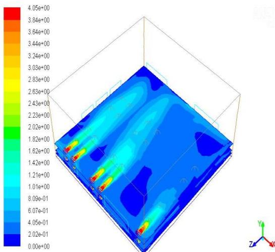
**Fig.12: Contours of velocity magnitude for Basic Case1 at y-plane.**
