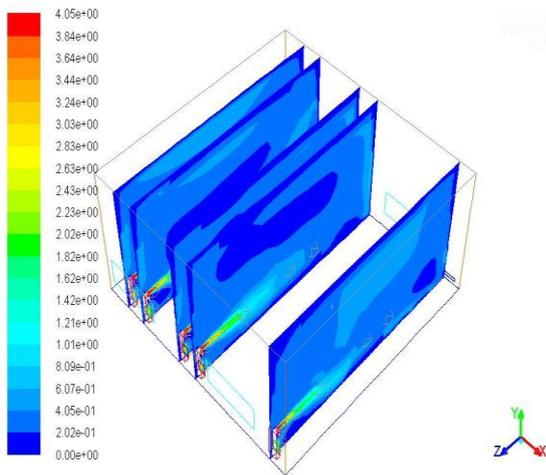
**Fig.10: Contours of velocity magnitude for Basic Case1 at x-plane.**
