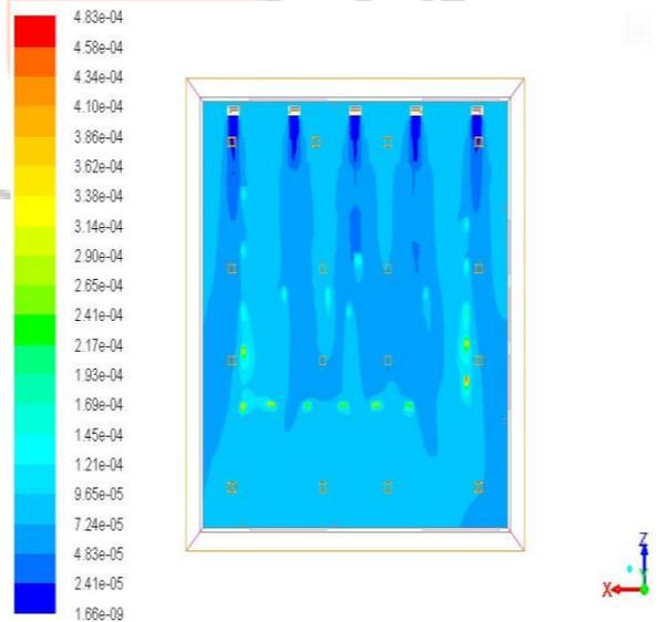
Fig.27: Contours of Co2 concentration for Case 2 at x-z plane.
