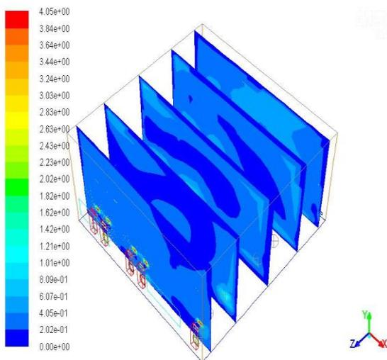
**Fig.11: Contours of velocity magnitude for Basic Case1 at z-plane.**
