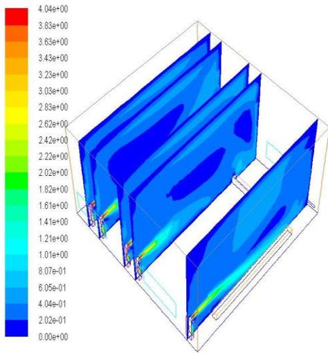
**Fig.16: Contours of velocity magnitude for Cooling Case1.**
