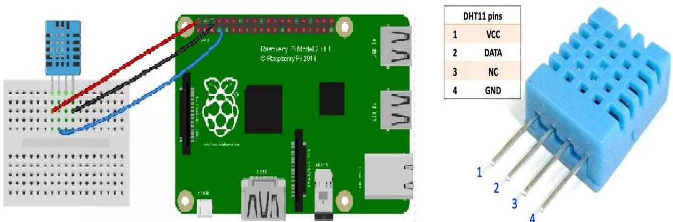
Figure 5: DHT11 with raspberry pi
