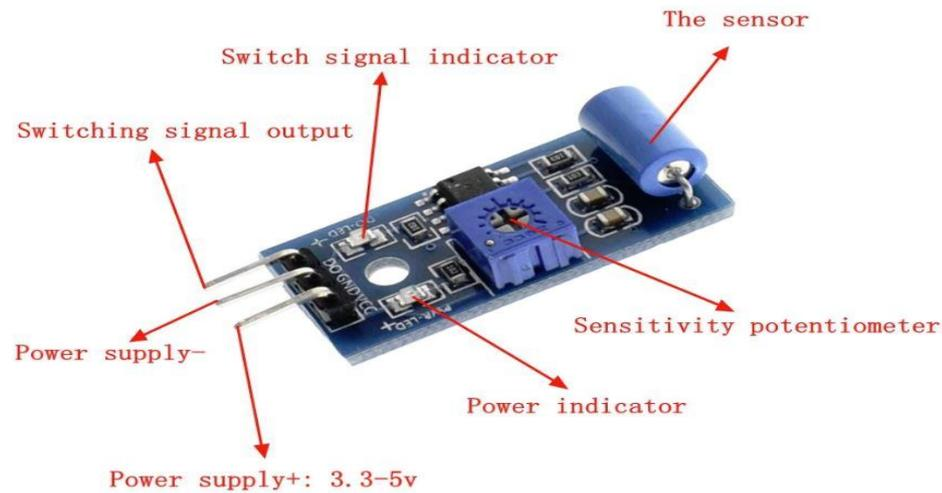
Figure 4: SW420 Vibration Sensor pin diagram
