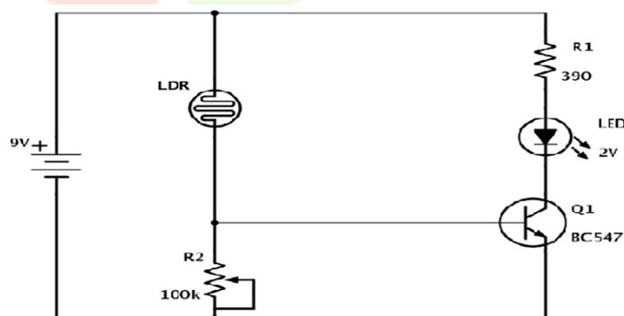
Figure 3: circuit diagram of LDR
