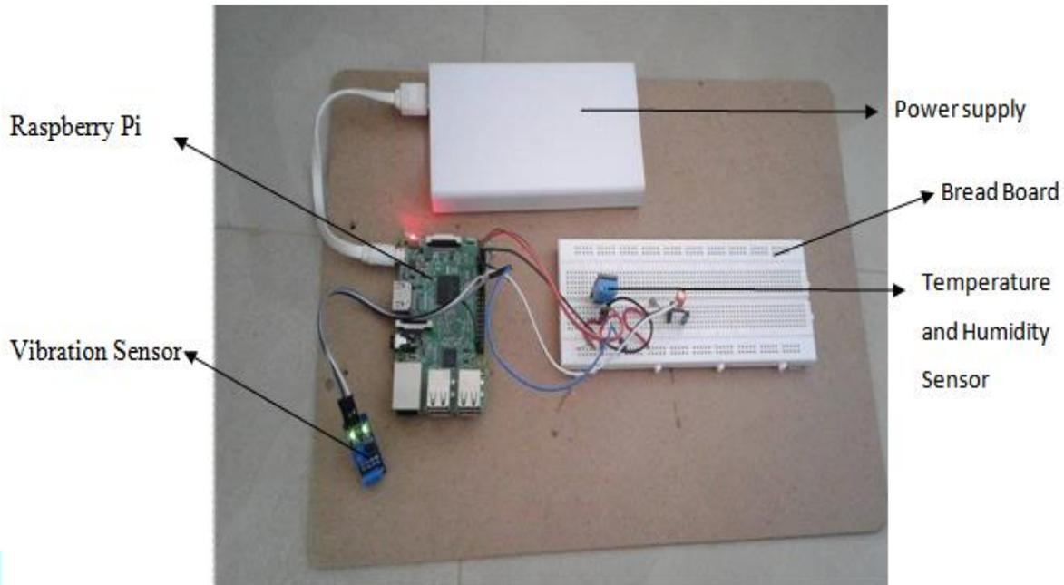
**Figure 8: Working Experimental setup for WSN**
