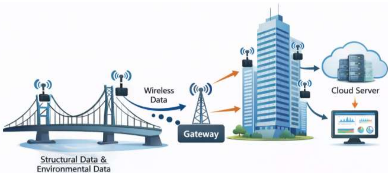
Figure 2.2: Wireless Sensor Network Deployment on a Structure
