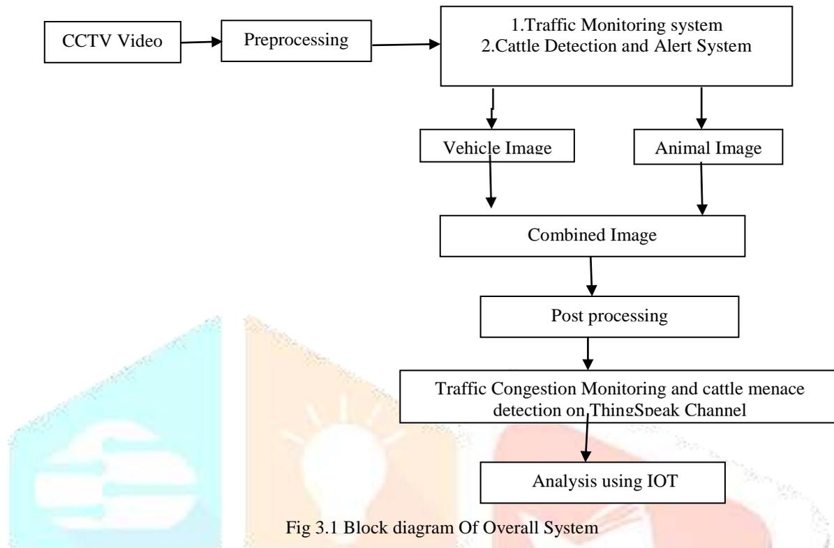
Fig 3.1 Block diagram Of Overall System
