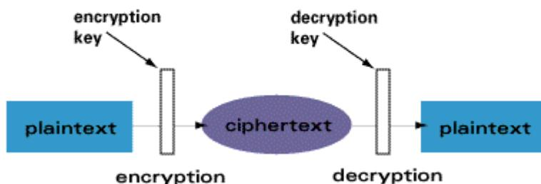
In general, symmetric algorithms execute much faster than asymmetric ones. In real applications, they are often used together, with a public-key algorithm encrypting a randomly generated encryption key, while the random key encrypts the actual message using a symmetric algorithm. This combination is commonly referred to as a digital envelope.
