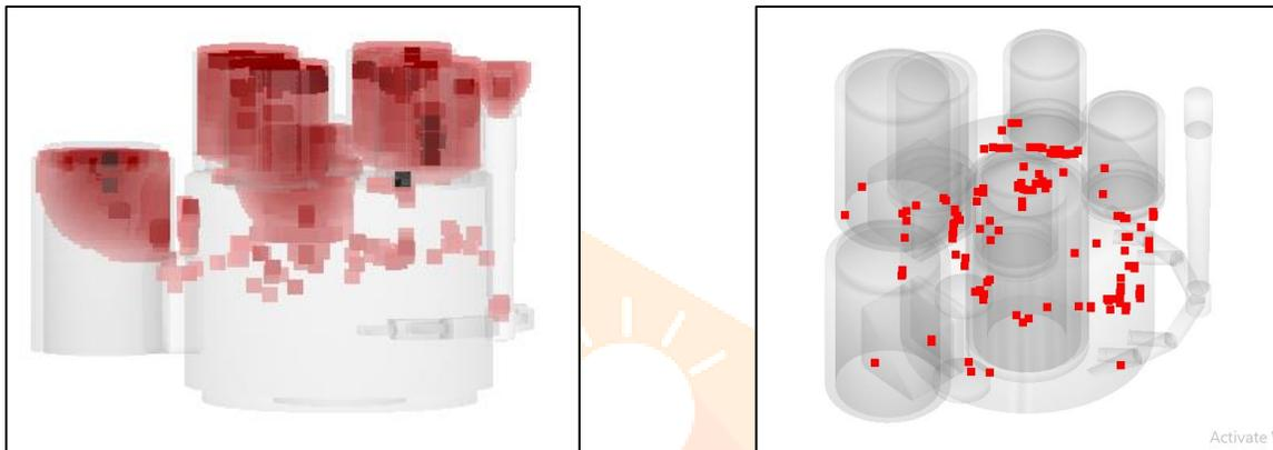
Fig: 4 (a) Chances of Shrinkage-Porosity in Casting (b) Chances of cold shuts
