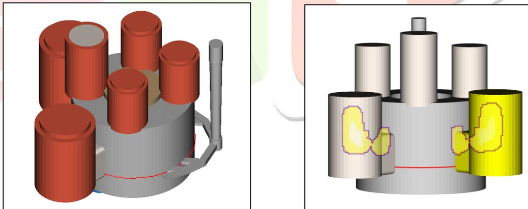
Fig: 3 3D model of gating system with simulation result.
