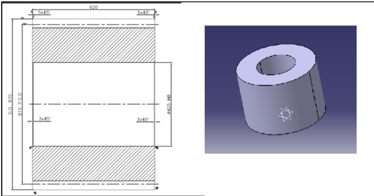
Fig: 2 Part Drawing and 3D model.
