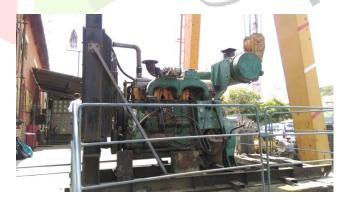
It is a 6-cylinder generator with two inlet and two outlet. Both the valves are generally Connect with centrifugal pump for high suction of crude oil. There are mainly two types of pumps, which are useful in crude oil suction gear pump, and Reciprocating pump both pumps are useful for land oil suction rig. In addition, centrifugal pump is useful for crude oil suction in ocean rig.
