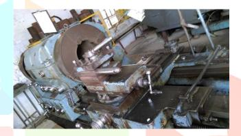
It is Russian manufactured machine with two side chalks but Final settlement of work peace is manual by workers. It is mainly use for big & heavy work pieces generally for threading and other operations for instance Internal & external thread. It also require some Extra supports for long pipe holding.
