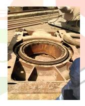
It generally settled near to dock head. It is main part for drilling rig .it is useful to transfer rotary motion from top head to bottom drill beat. From one side electrical or mechanical energy provide according to rig and by that energy rotary motion take place, complex Gear system is available inside the table.
