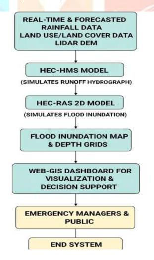
The process begins with inputting Quantitative Precipitation Forecasts (QPF) into the calibrated HEC-HMS model, which generates a predicted streamflow hydrograph at critical points. This hydrograph is then used as an input boundary condition for the 2D HEC-RAS model, which calculates how the water will flow across the floodplain, producing detailed maps of flood extent and depth. These maps are finally disseminated via a user-friendly dashboard.
