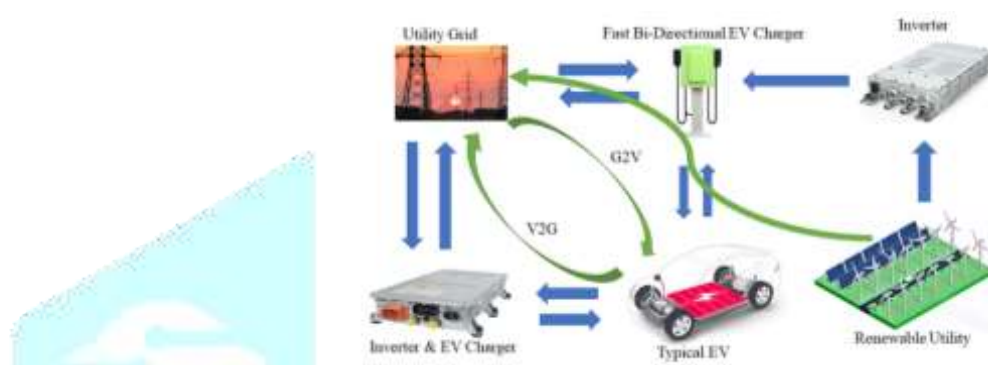
Fig 1: Block diagram of G2V and V2G power flows between electric vehicles, chargers, the grid, and renewable sources (adapted from [Source]).
