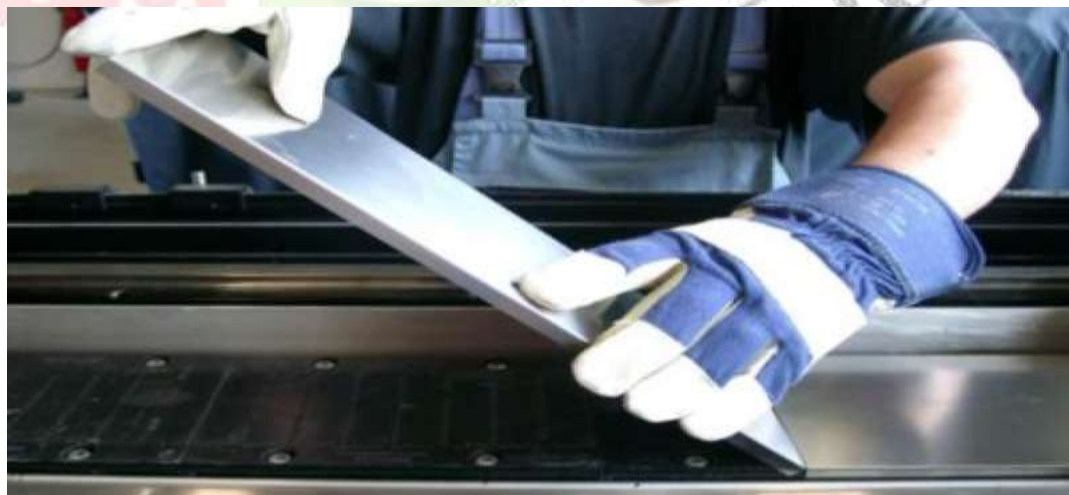
Fig. 22 Mounting of a further segment of the segmented secondary section cover
