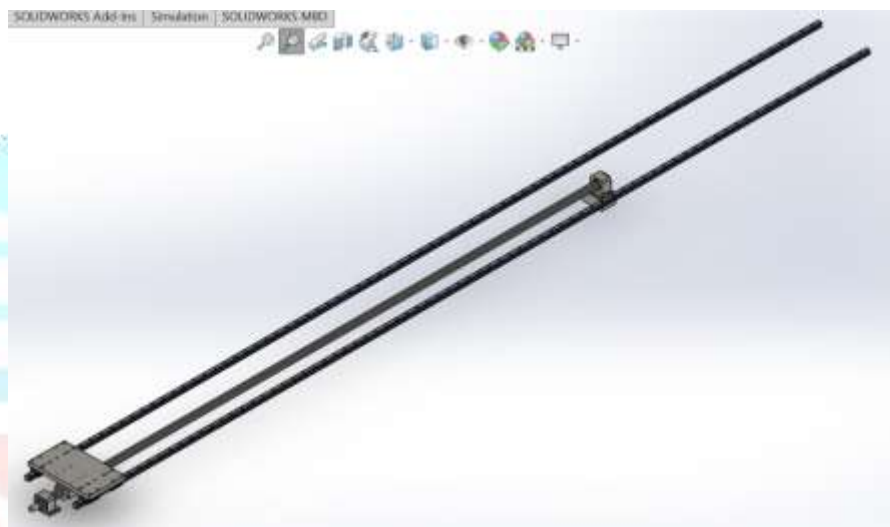
Fig. 9 3 D Model of Ball Screw Mechanism for XYZ axes of Fibre Laser Cutting Machine
