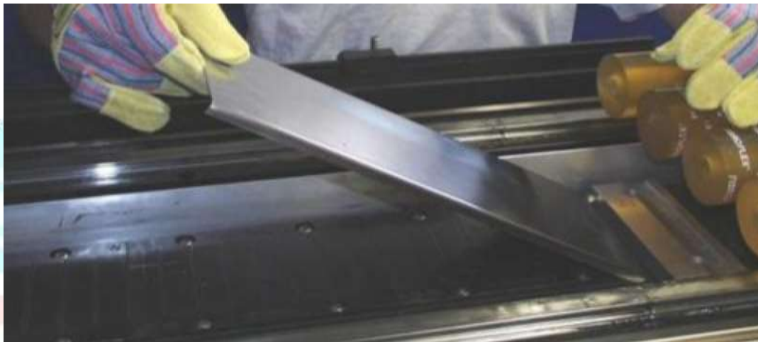
Fig. 21 Mounting of the first segment of the segmented secondary section cover
