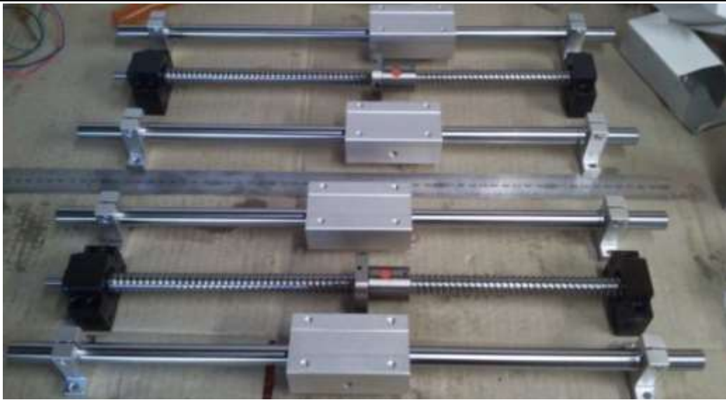
Fig. 8 Real Image of Internal Ball Return System for CNC axes
