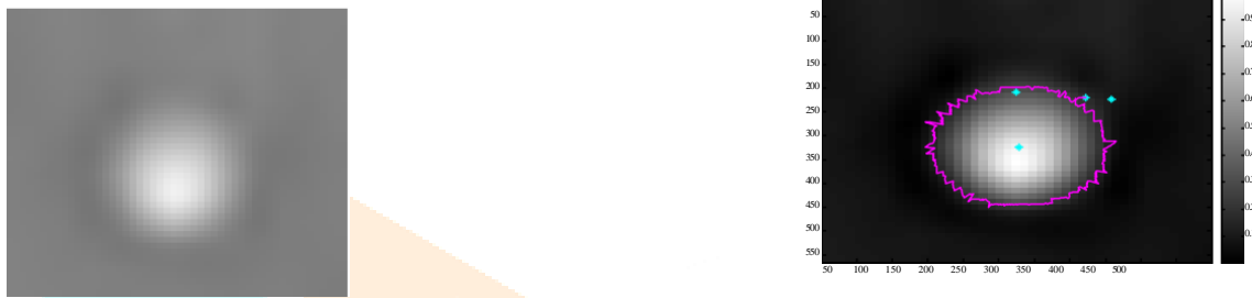
Fig.3. a) A horizontal slice of a C-scan, acquired at 1.39 nsec after the GPR signal emission [7];
