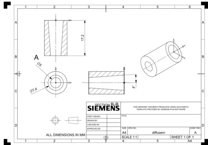
Where  $D_1$  is the inlet diameter of the diffuser = 5 mm
