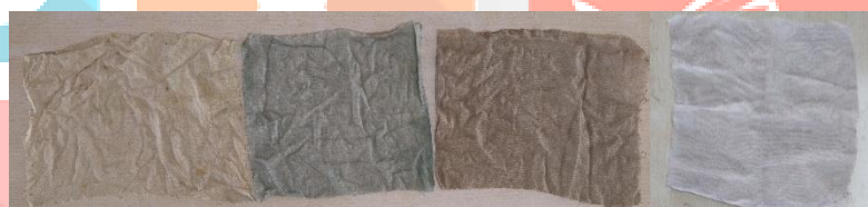
Figure 4 : dye fastness on fabric samples after washing : 1 st fabric(sodium carbonate), 2 nd fabric(copper sulfate), 3 rd fabric(ferrous sulphate) and 4 th fabric(alum)
