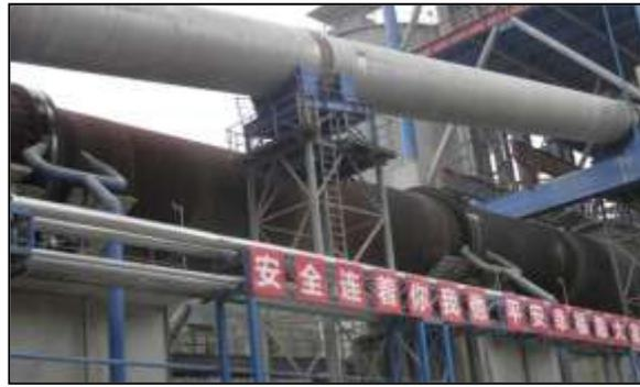
Figure no.5 Rotary kiln in a cement plant of China.
