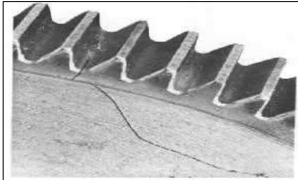
Figure no.7 failure by cracking
