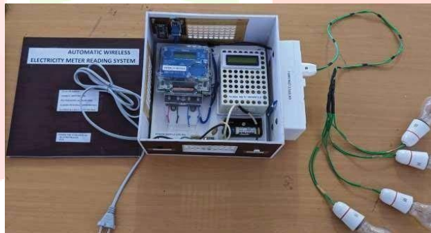
Fig.6. Working model of IOT Based Automatic wireless Electricity Meter Reading System
