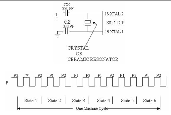
Oscillator and timing circuit
