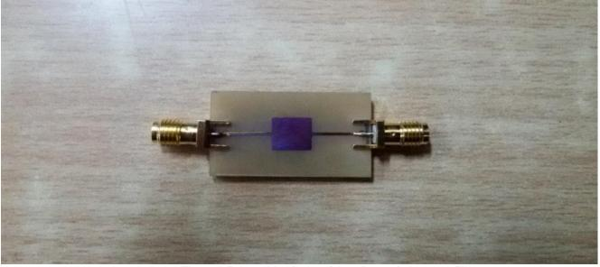
Figure 5: Prepared hardware of the micro-strip low pass filter
