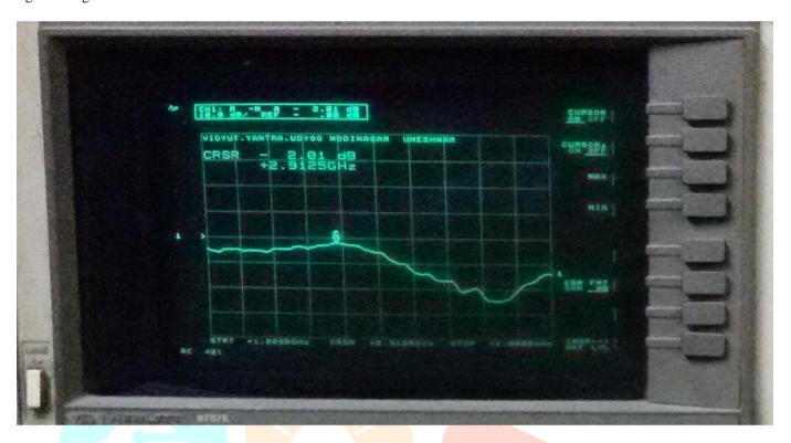
Figure 6: Response of third order stepped impedance micro-strip low pass filter (insertion loss) using network analyzer
